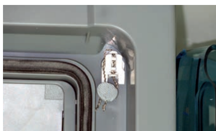
Sealing the screws on the front panel
