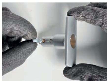
Insert the pin in the notch towards the front
