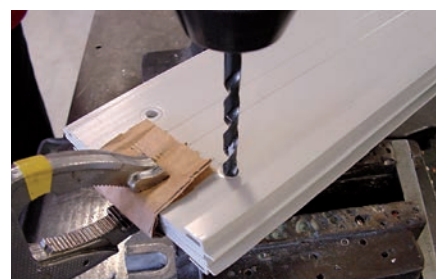
Drill both sides at the same time (Ø 6.5 mm)
