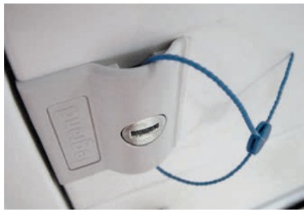
Sealing the faceplate in locked position
